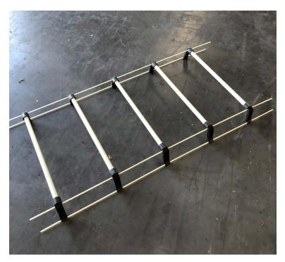
**Fiber dowels baskets** are made of biomaterials and fiber glass. Pavement specifications typically include placement tolerances. These tolerances call for dowels to be placed reasonably close to parallel with the pavement centerline and the pavement surface.
